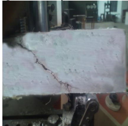
Fig. Crack Pattern of Beam Failed in Shear
